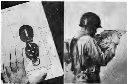
Figure 26. Orientation of map by compass.
